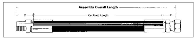
For most assemblies, the correct assembly length may be determined by direct measurement of the equipment or a drawing. Minimum bend radii as shown in the hose specification tables should be observed.
