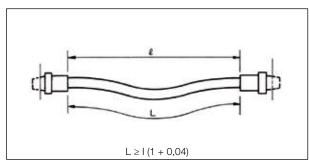
Occasionally an assembly will be required similar to the sketches to the right. The following equations are helpful in determining the correct length:
