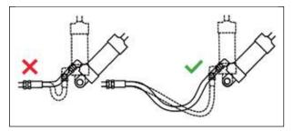
Adequate hose length is most important to distribute movement on flexing applications and to avoid abrasion.
