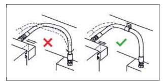
To avoid twisting in hose lines bent in two planes, clamp hose at change of plane, as shown.
